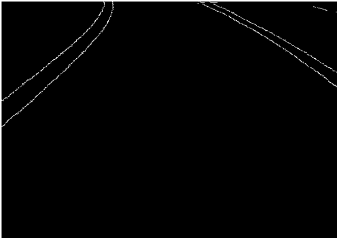
Fig 6: Left – Edges detected through Canny edge detection algorithm after making required changes. Right – The input image for Canny edge detection algorithm.
